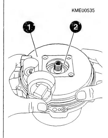
ASSEMBLING ALTERNATOR Fitting cap Secure new cap (1) with new bolts (2). Fasten connection/terminal B+ (3). Use new nut. Use torque wrench. Tightening torques Ball-bearing retaining 7,0...7,6 Nm plate: 18...22 Nm Terminal B+: comm. avail. Torque wrench: comm. avail. Torx T25:
